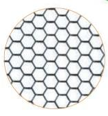
The 81 % open honeycomb structure enables turbo heat development and shorter baking times.
